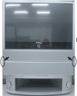
Remove the screws on the left/right
